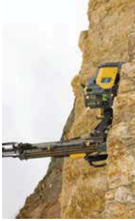
The FlexiROC D60 is built for high efficiency mining. Its DTH hammer benefits from a precisely matched compressor.
